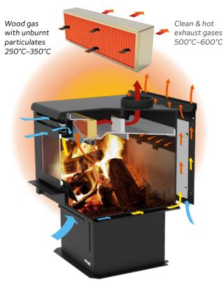
The catalytic combustor helps create a controlled flame that allows a more even burn rate helping to:
