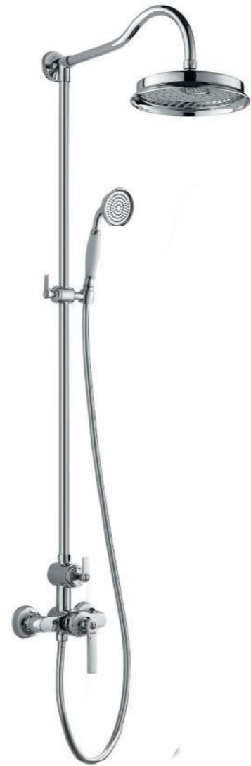
FWL7629CP Shower tower and mixer with 1 spray function handshower, chrome 1150mm high x 720mm reach WELS 0 star (10 L/min regulator included)
