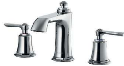
FWL8259CP 3 hole deck mounted basin set, chrome 90mm aerator height x 130mm reach WELS 3 star 8L/min
